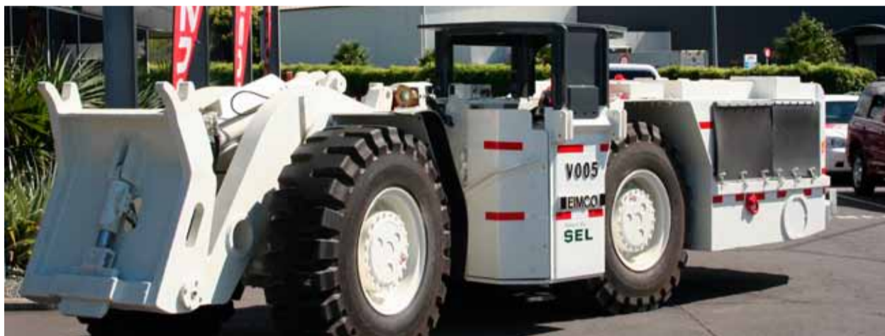
An Eimco ED7 underground wheel loader with a quick attachment handler. (Now operating underground at Solid Energy's Huntly East mine)
